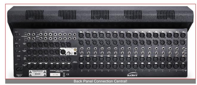
Parallel processing is possible on every channel strip through use of the always-active channel insert send output. This would connect to a processor input, with the returned processed audio routed to the Alternate input path to be summed with the original signal into the stereo mix bus.
