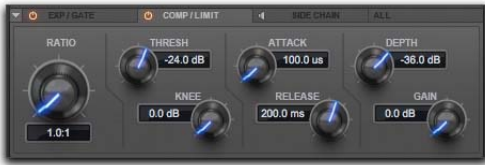
Dynamics section, Compressor/Limiter tab
