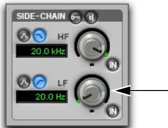
LF frequency controls
