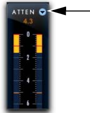
Output/Attenuation toggle, Attenuation meters shown
