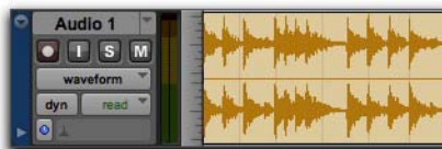
Track View set to Waveform for audio track
