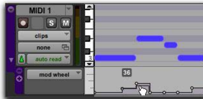
Stepped control automation
