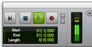
Output meters in the Transport window
