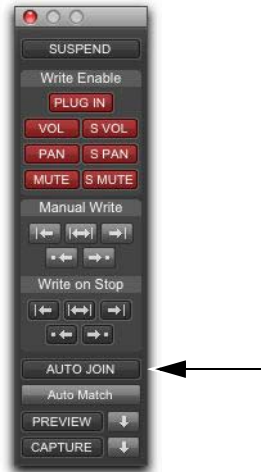
AutoJoin Enable button in the Automation window
