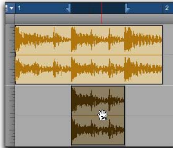
Dragging to another track with the Separation Grabber tool
