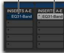
Indication of bypassed plug-in state
