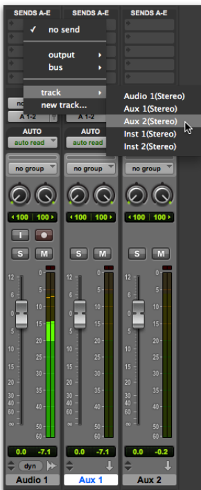
Assigning a send to an existing Auxiliary Input track
