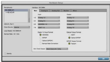
Hardware Setup for HD OMNI, Main page
