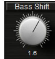
The Bass Shift is an „intelligent“ EQ band for the bass frequencies of your mix. We call it Bass Shift because 2 different frequencies will be „shifted“ against each other with the turn of just one knob. The frequencies have been pre-set and cannot be changed. If you are looking for a sweepable Bass- (and Presence-) Shifter please check out bx\_hybrid (available individually).
