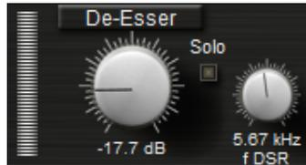
The bx\_digital De-Esser works with dynamic EQs that you can adjust to the needs of your mix. With the Solo button of the De-Esser section it is possible to listen to only the frequencies that you want to filter out of your mix.
