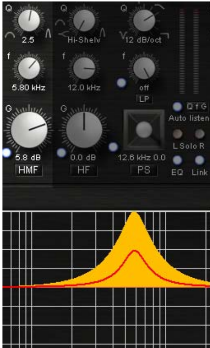
Auto listen "Q" with positive gain (see the HMF band gain at (+5.8dB))
