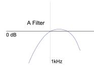
Choose **Filter A** from the dropdown list to apply A-weighting to your RMS measurements. A-weighted signals are usually indicated by the unit dB(A) or dBA. It is based on the 40-phon Fletcher–Munson curve, which means that it refers to the human ear reception on quiet sounds. It emphasizes mid frequencies between 1 and 6 kHz and attenuates low and high frequencies (see picture).
