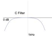
**Filter C** applies C-weighting to your RMS measurements. C-weighted signals are usually indicated by the unit dB(C) or dBC and are based on the 90-phon Fletcher–Munson curve, which means that it refers to the human ear reception on loud sounds. It passes through a broad mid frequency band and attenuates low and high frequencies (see picture).
