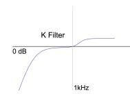
**Filter K** applies K-weighting to your RMS measurements. This filter follows the ITU-R recommendation BS.1770-1 and emphasizes high frequencies above 1 kHz while attenuating low frequencies below 200 Hz (see picture). Don't confuse the K-Filter with K-Metering explained in Chapter 4.5.2. It is not the same.;)
