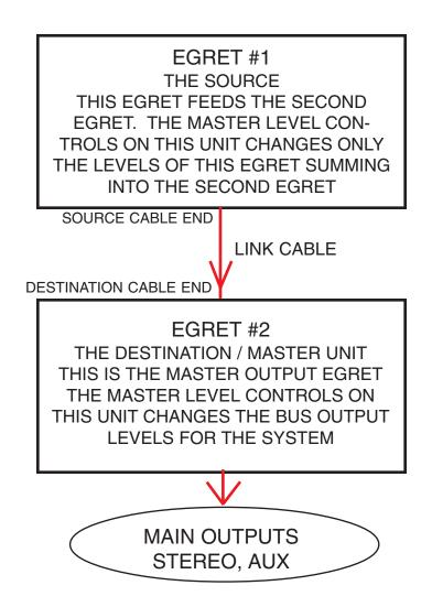
In ths configuration each of the two Egrets has 8 digital / analog inputs for a total of 16 inputs. Linking the units together works by tieing the summing bus inputs to the approate outputs. The source and destination units are select by how the link cable is plugged in.
