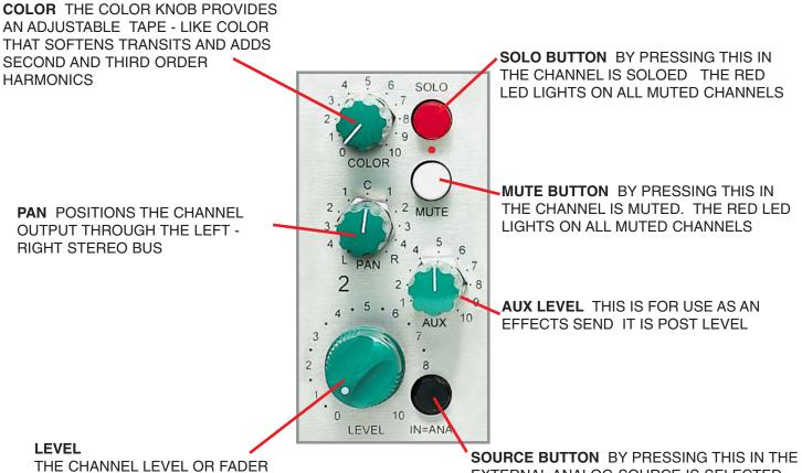
SOURCE BUTTON BY PRESSING THIS IN TH EXTERNAL ANALOG SOURCE IS SELECTED. WITH IT OUT THE CHANNELS D/A CON-VERTER IS SELECTED
