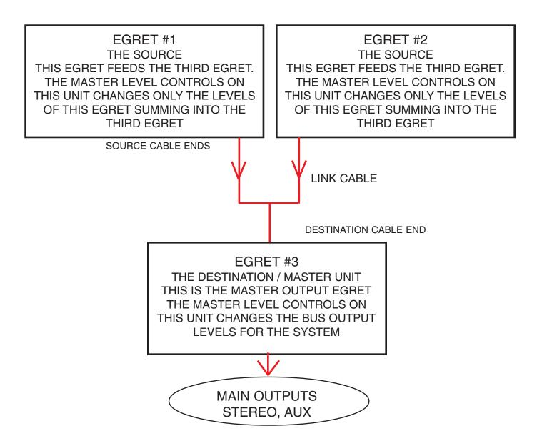
In ths configuration each of the three Egrets has 8 digital / analog inputs for a total of 24 inputs. Linking the units together works by tieing the summing bus inputs to the approate outputs.
