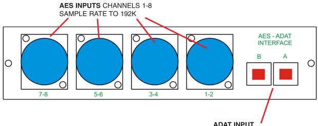
ADAT INPUT INPUT A IS THE 48K INPUT INPUT B IS THE SECOND SET OF CHANNELS IN THE SMUX MODE
