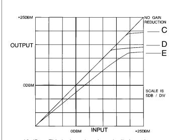
**Graph C** shows the limiter input/output gain relationship with **no** compressor operation. The Pk Threshold is set at +19 dBm. The graph shows a maximum gain reduction of 6db when the input is at +25 dBm.
