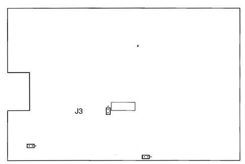
If you do this the unit MUST BE FIRST BE DISCONNECTED FROM AC POWER, THE CORD UNPLUGGED. You should ground your self to the unit before removing the top cover and remain in physical contact with the unit to prevent static discharge. If you are unsure get a tech. to change the jumper.
