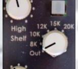
20kHz Low Pass Filter 6DB per Octave
