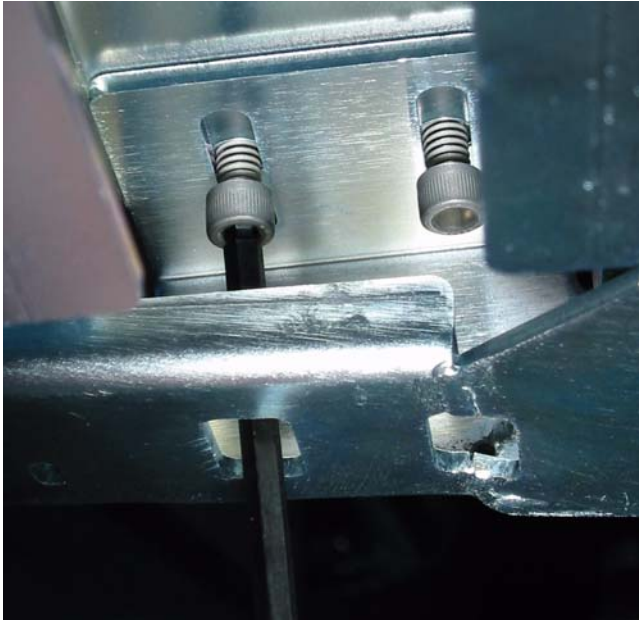
Figure 13. Attaching support rail from below
