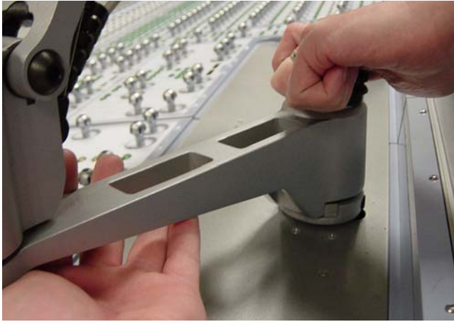
Figure 40. Placing the arm assembly on the mounting post
