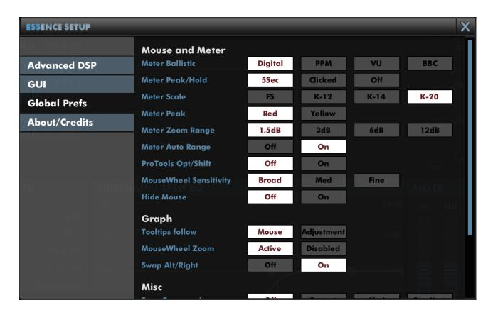
Meter Ballistic allows you to pick the ballistics used by the meters.
