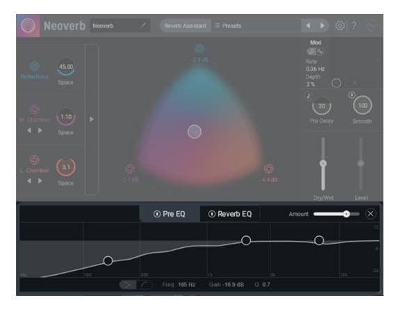
Neoverb has two 3-band EQ modules, one before the reverb (Pre EQ), and one after (Reverb EQ). EQ before and after reverb can optimize the overall sound, as described below.
