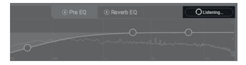
4. Neoverb shows a suggested EQ curve after completing its analysis. The Amount slider scales the amount of cutting EQ. The higher the number, the greater the cut.
