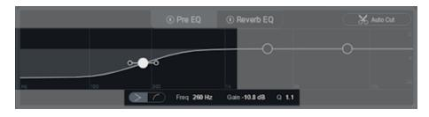
• The **Low-Cut** shape progressively attenuates the audio level below the selected frequency. The EQ node handles set the slope, or how rapidly the audio level falls off below the selected frequency. The slope options are 6, 12, 24, and 48 dB/octave. Note that the filter can only attenuate, not boost, with this shape.
