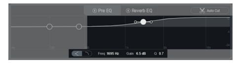
• The **High-Cut** shape progressively attenuates the audio level above the selected frequency. The EQ node handles set the slope, or how rapidly the audio level falls off above the selected frequency. Note that the filter can only attenuate, not boost, with this shape; the image shows a cut with a 6 dB/octave slope, starting at 1,695 Hz.
