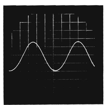
This unretouched photo shows the acoustic output of the system when driven by a 50 Watt sine wave signal at 35 Hz. A laboratory microphone was used to pick up the sound from Model 4310. The signal from the microphone was connected directly to an oscillo-scope and the trace photographed.
