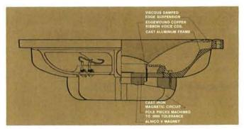
Section drawing of 12-inch low frequency transducer.
