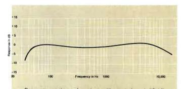
Response contour of system with controls set "flat." (Presence set at "2," Brilliance set at "7.") Measured on-axis response of a typical 4310, including
