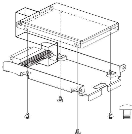
4. Slide the Tray with Hard Disk Drive into the slot and press it firmly to ensure secure connection. Tighten the two screws back that have been removed in Step 2. Place the Front Cover back and tighten the four screws back that have been removed in Step 1.
