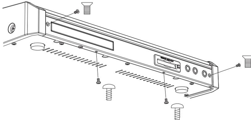
2. Remove the two screws for Internal Hard Disk Drive Tray and remove the Tray with your fingers at the
