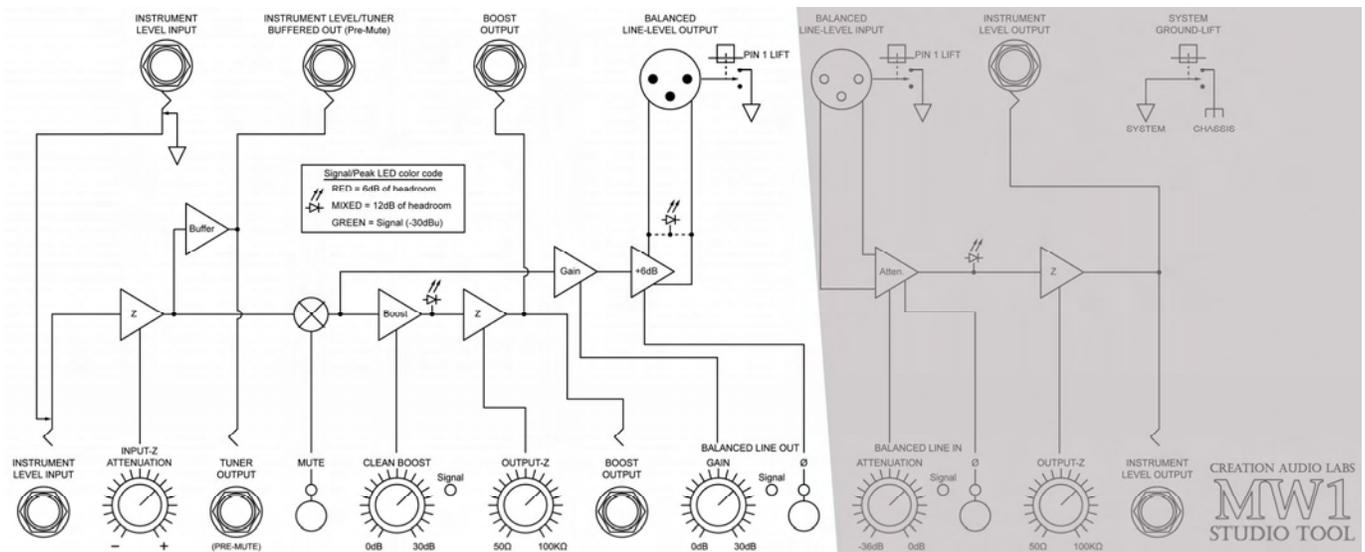
\*\*\*All 1/4” jacks are duplicated on the front and back of the MW1 Studio Tool. With the exception of the **INSTRUMENT LEVEL INPUT** connections, all 1/4” jacks front and back will be active at the same time. As such, the duality of the output jacks allows for multiple signal path routing. The **front INSTRUMENT LEVEL INPUT** takes priority over the rear input.
