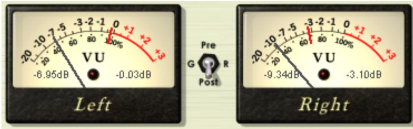
PSP MasterComp meters are designed to both look and operate similarly to hardware VU and PPM meters with overs indicators. To ensure that these meters will be a useful tool in every situation we endowed them with enough parameters to allow you to adjust the meters' behavior to nearly any practical situation. To learn more about those adjustable parameters read the **Rear Panel** section of this manual.
