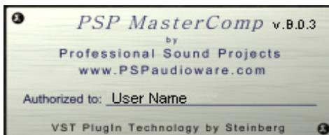
The Plug-in Information plate consist of the version number of the plug-in to the right of the plug-in name, and your authorization details. Clicking anywhere in the Plug-in Information Plate switches the GUI back to the front panel.
