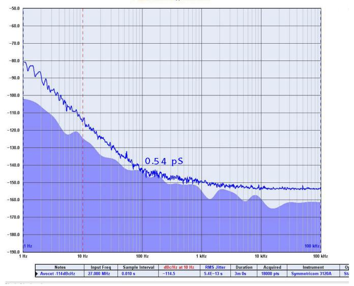
Jitter measured from 1Hz to 100KHz is 0.54pS typical.
