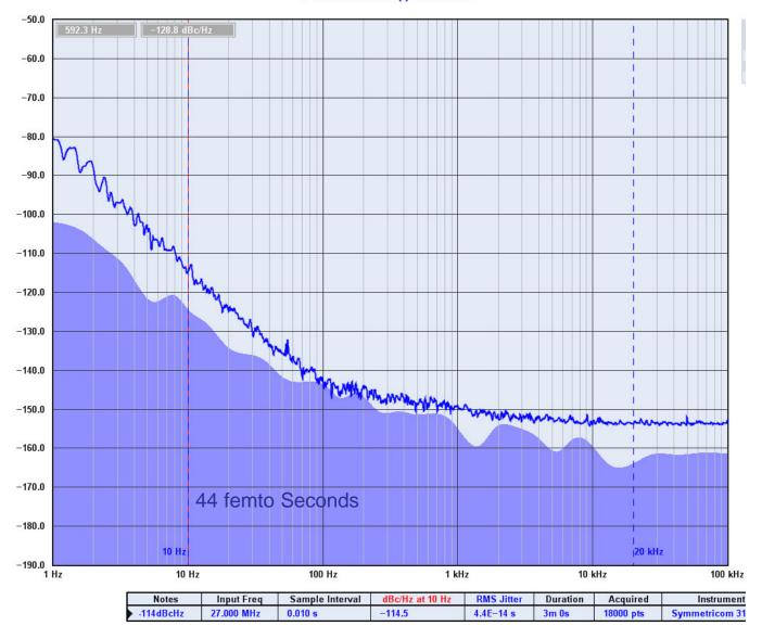
Jitter measured from 10Hz to 20KHz is 0.044pS or 44 fS typical.
