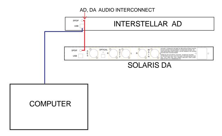
By using the AD as the master interface the clocking will be uncompromised For playback only SOLARIS can connect directly to the computer by USB
