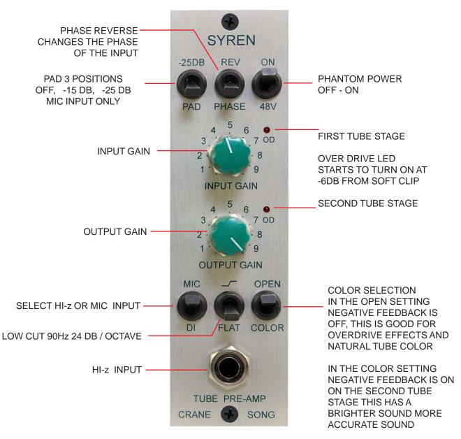
HOWEVER THE FINAL SOUND WILL BE DETERMINED BY THE SETTINGS OF THE GAIN CONTROLS, THE COLOR SWITCH AND THE SOURCE IMPEDANCE, EXPERIMENT A LITTLE. SETTING THE OUTPUT GAIN TO MAX WILL BE CLEANER, SOFT OVERDRIVE MORE COLORED.
