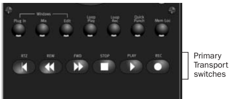
Command|8 Transport controls
