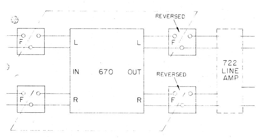
THE FADERS MARKED "F" ARE GANGED 20 STEP - 20 DB "T" ATTENUATORS
