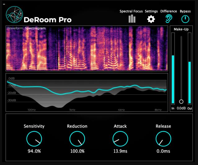
At the top right of the plugin you will find four buttons: Spectral Focus, Settings, Difference and Bypass.
