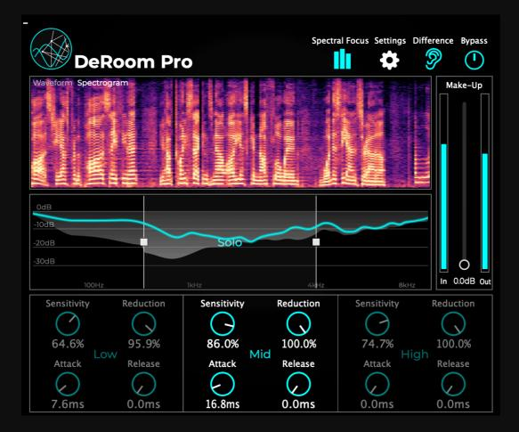
You can adjust the cutoff frequencies by dragging the squares in the gain view. By clicking a band it can be played in solo which lets you adjust the reduction controls for each band separately.
