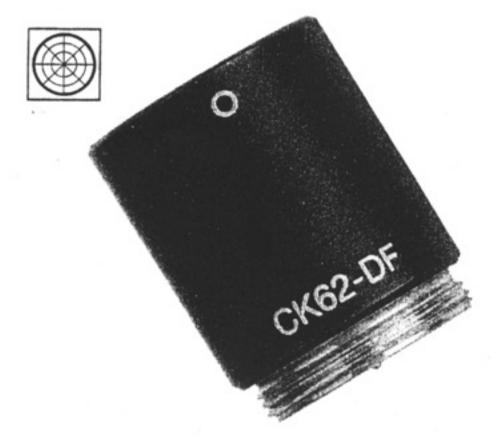
Omnidirectional capsule with specially equalized frequency response. For far-field miking outside the room radius, where most of the sound arriving at the microphone is reflected, diffuse sound.
