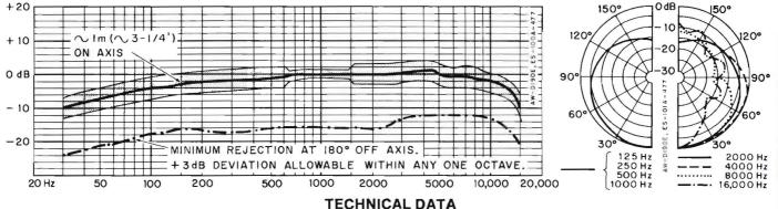
Transducer Type: Dynamic Directional Characteristic: Cardioid Frequency Range: 30-15,000 Hz Nominal Impedance: 200 ohms
