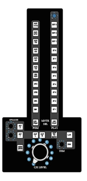
The Control Room Monitor Select (MNTR SEL) section allows the choice of Program and Playback monitor sources and contains the main Control Room monitor level control.
