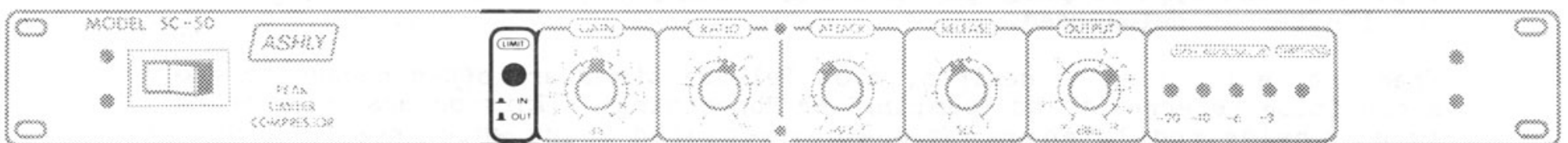
Figure 16 When the LIMIT switch is in the OUT position, all limiting and compression effects are by-passed. For normal operation, the switch should be IN.
