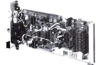
DA100 Basic One In, Six Out Distribution Amplifier. Single power stage drives six active balanced outputs at +22dBm each. Split and by-passed build-out resistors give protection against shorts and RF. Balanced bridging input. Single panel level control sets all outputs. Headphone monitor jack
