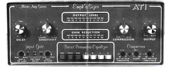
The Emph' a Sizer COMPRESSOR is designed around a pro-audio, monolithic, 100 db range, low noise VCA. High headroom capability allows the VCA to handle maximum inputs without input attenuation and thereby achieve maximum signal to noise performance on low level inputs
