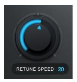
Retune Speed controls how rapidly the pitch correction is applied to the incoming audio. A zero setting will cause immediate changes from one pitch to another, and will completely suppress any vibrato or deviations in pitch.
