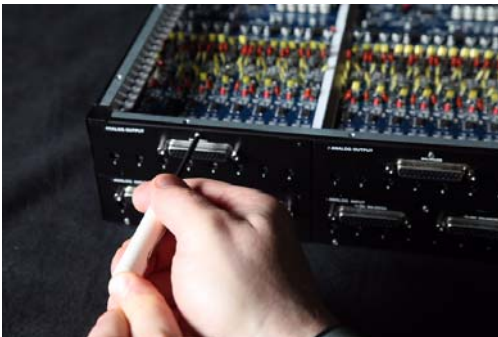
Removing the screws securing an I/O card
