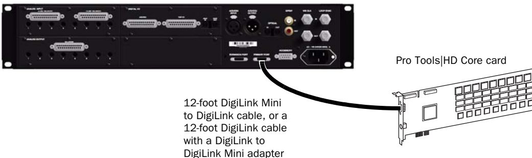
Figure 1. HD I/O connected to the DigiLink Port on a Pro Tools|HD Core card (16-channel I/O system)
