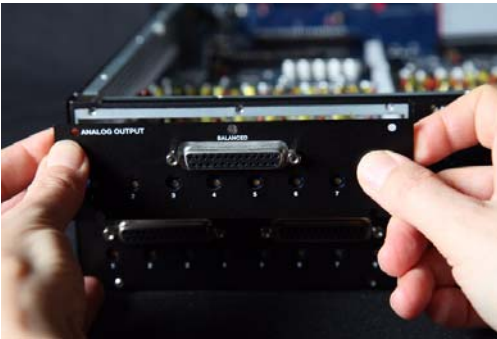
Lifting slightly while pushing the card back into the bay
