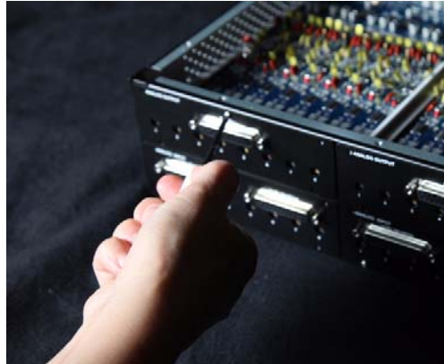
Securing the I/O card to the back panel of the HD I/O
