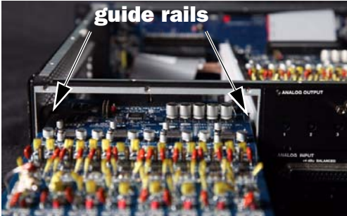
Inserting the card into the guide rails for the empty bay
