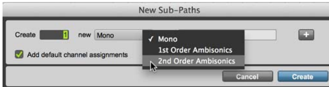
Selecting a 2nd Order Ambisonics sub-path for a 3rd-order Ambisonics path
