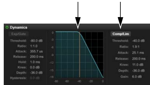
Dynamics, Exp/Gate disabled and Comp/Lim enabled
