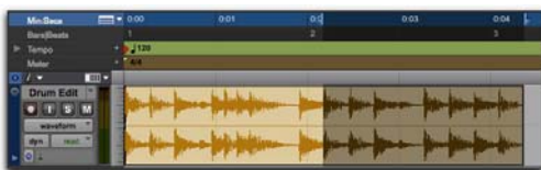
Making an audio selection for Beat Detective
