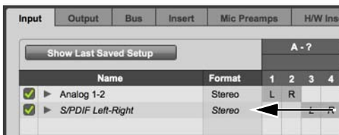
Unavailable hardware Input shown in italics
