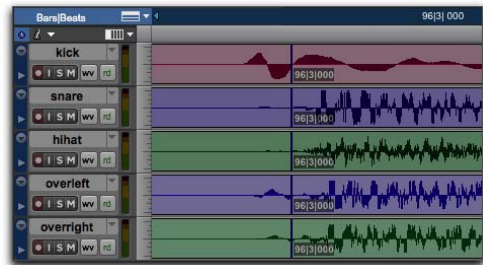
Overhead mics generate late beat triggers
