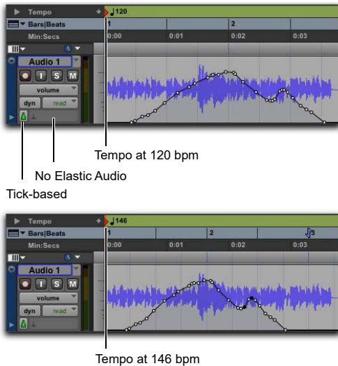
Tempo change applied to long sampled-based audio clip on a tick-based track, showing automation drift
