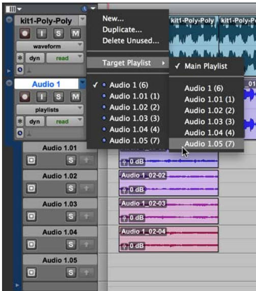
Designating the Target Playlist for a stereo audio track
