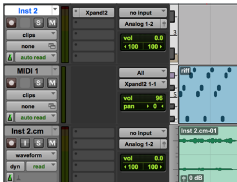
Source MIDI Track (middle) assigned to a Virtual Instrument plug-in on the Instrument track (top) and the Committed track (bottom)
