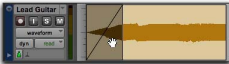
Selecting a fade with the Time Grabber
