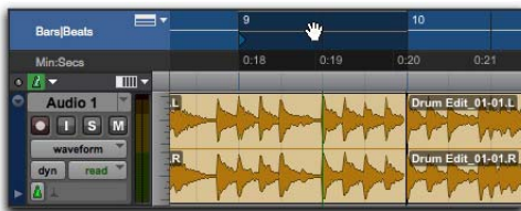
Dynamic Transport mode, moving the Edit selection
