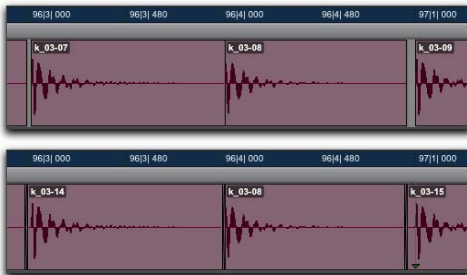
Clips before and after Edit Smoothing
