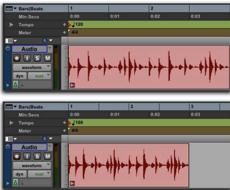
A clip group on a tick-based audio track at 120 BPM and at 160 BPM
