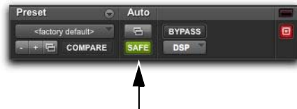
Automation Safe enabled plug-in
