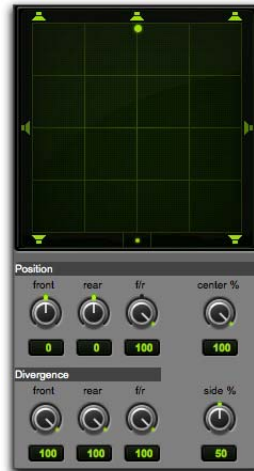
Side % set to 50% (side center speakers dimmed)
