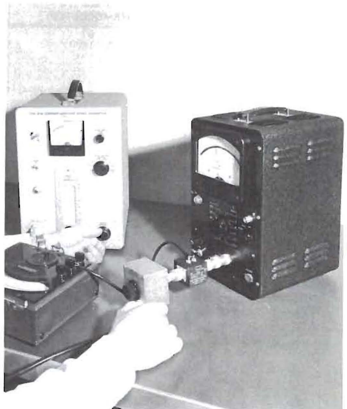
Model 440 Micropotentiometer being used to calibrate voltmeter on right.
