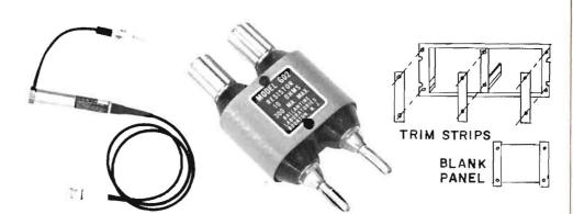
Model 1301 High Voltage 80d B Attenuator Probe for measurements to 10,000 Volts at frequencies up to 1MHz. Input impedance is greater than 10,000 megohms shunted by less than 4.5 picofarads. Shielded dual banana plug termination. \$90.
