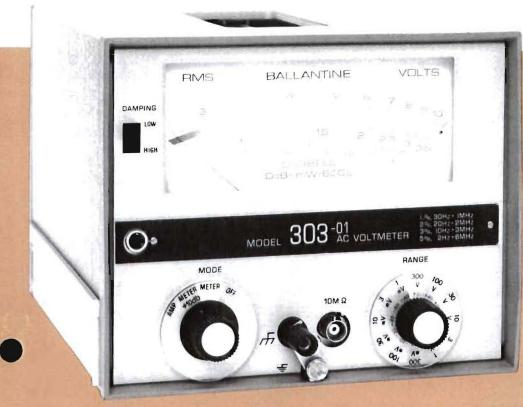
VOLTAGE RANGES: 300<sub>u</sub>V to 1000V FREQUENCY RANGES: 2Hz to 6MHz AVERAGE RESPONDING, CALIBRATED IN RMS OF SINEWAVE.
