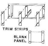
Model 800 Rack Mounting Kit for adapting one (or two) Series 323 voltmeters to a  $7'' \times 19''$  rack, without modification of the voltmeters. \$50.
