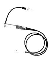
**Model 1301** High Voltage 80d B Attenuator Probe for measurements to 10,000 Volts at frequencies to 1MHz. Input impedance is greater than 10,000 megohms shunted by less than 4.5 picofarads. \$90.
