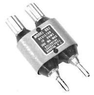
Series 600 Shunt Resistor Assemblies plug into input of Series 323 for measurement of current over a range of 0.1 microamperes to 10 amperes. Resistor values are in six decade steps from 0.01 ohm to 1000 ohms, thus making it possible to read current from the voltage scales.
