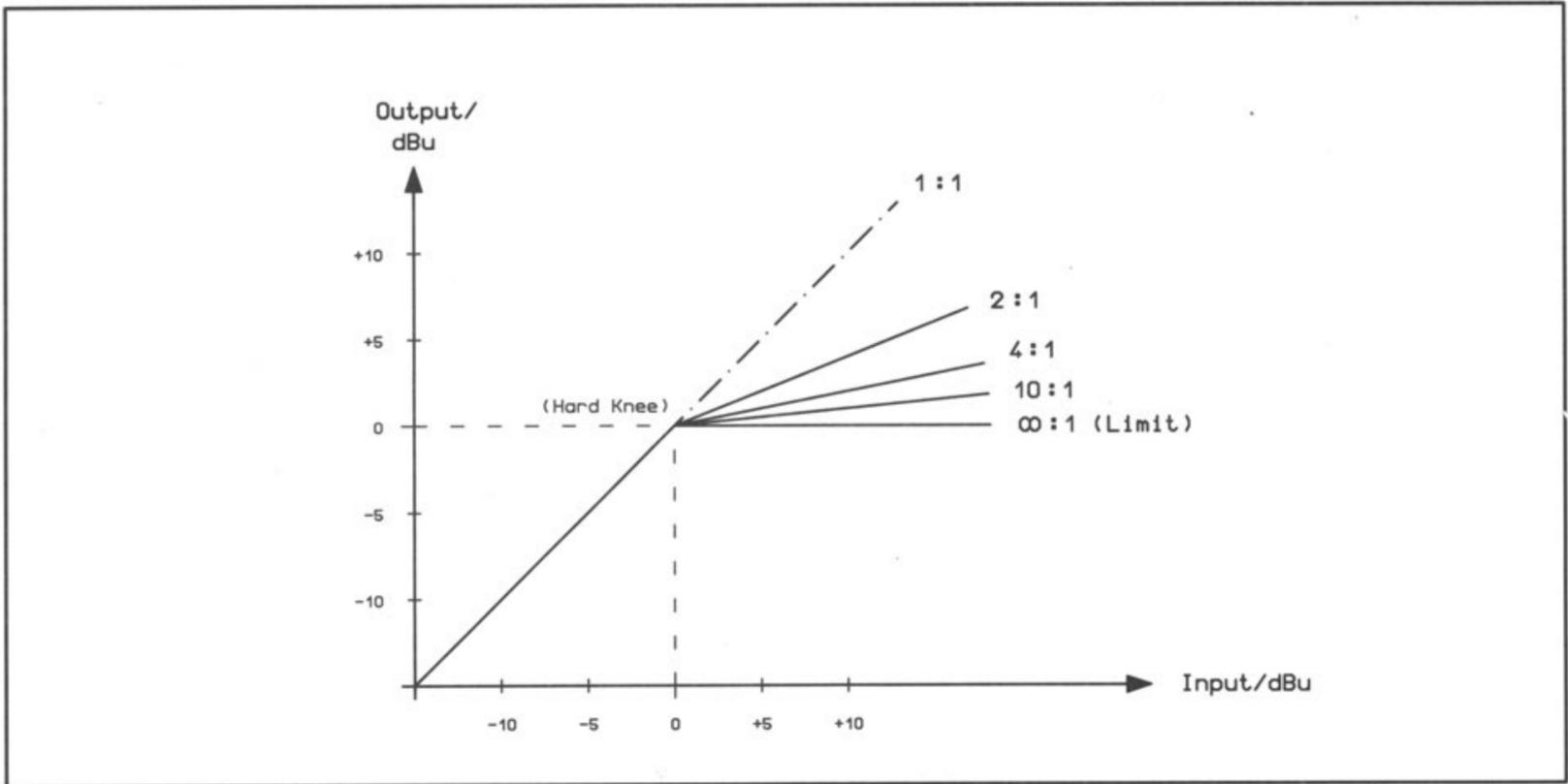
Fig. 18 The ratio of input to output level with reference to different ratio settings
