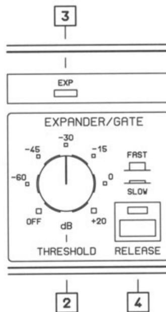
Fig. 12 Control surface of the Expander/Gate section
