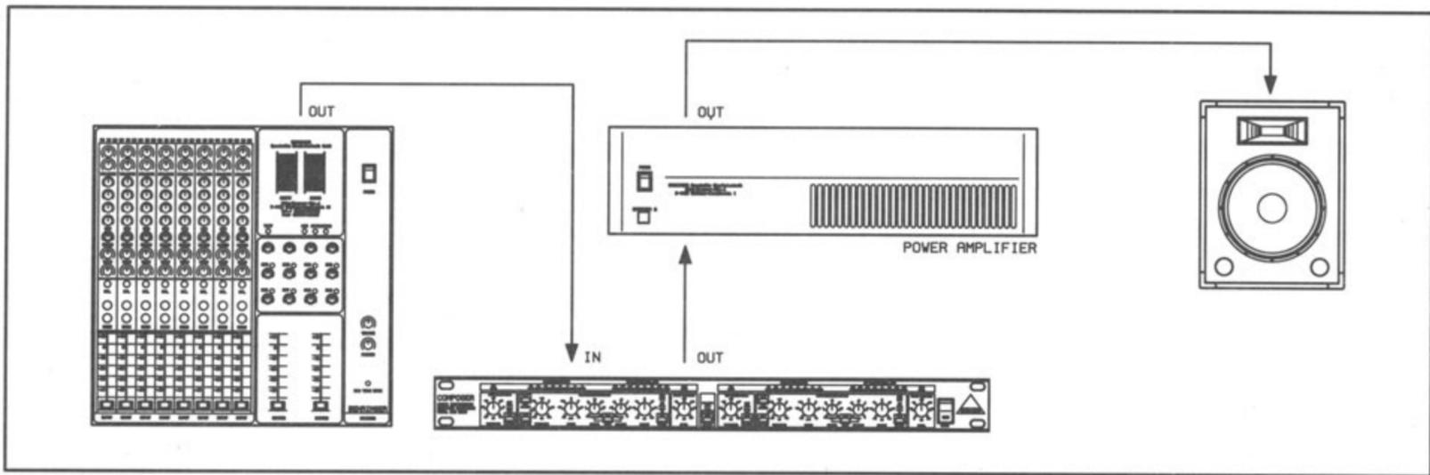
Fig. 30 Integrating the Behringer COMPOSER into a system with a passive crossover network
