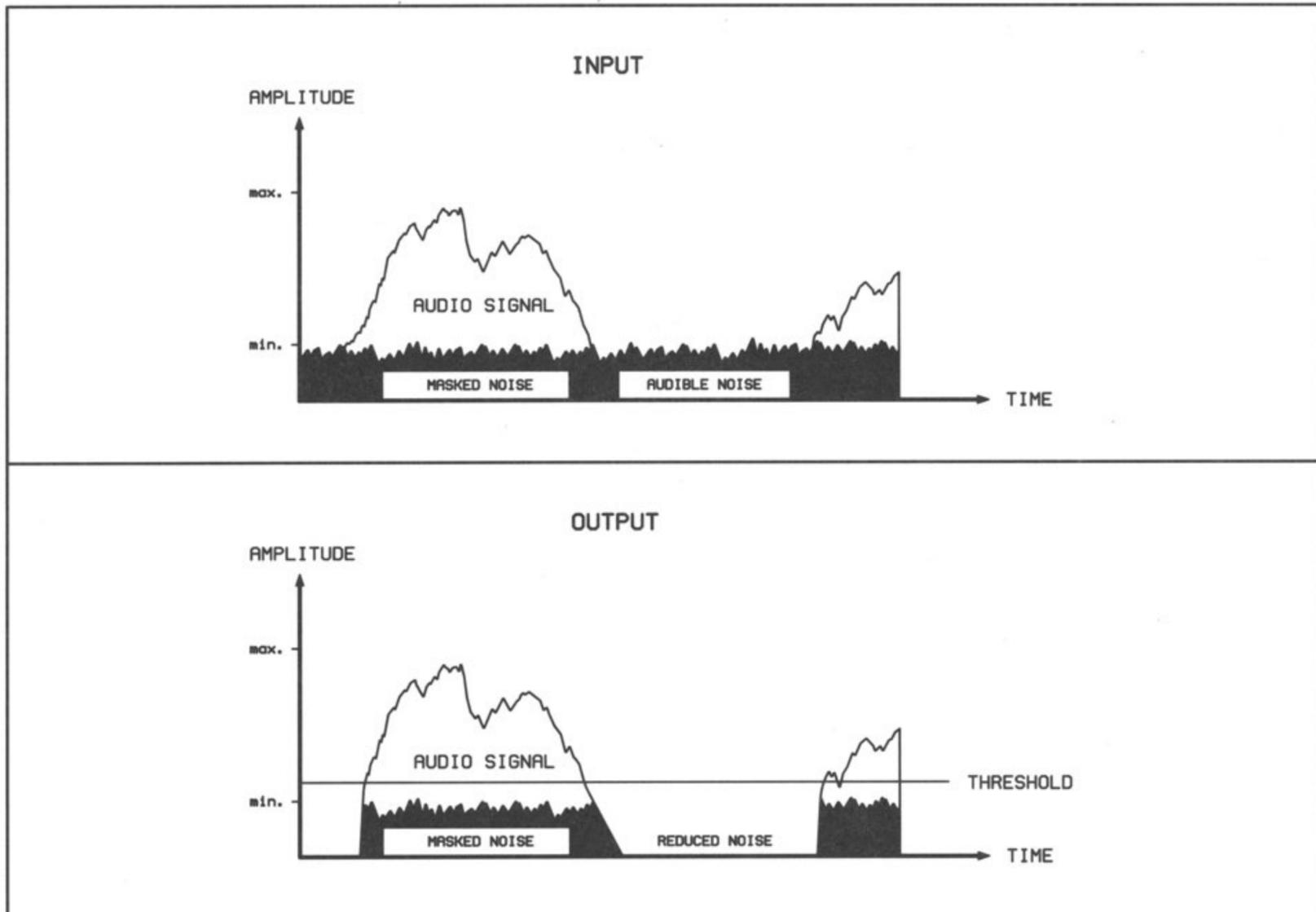
Fig. 16 Function of an expander
