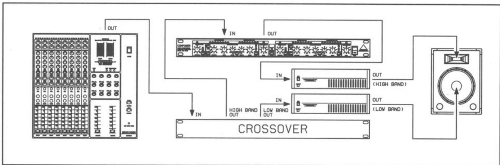
Fig. 32 Compressing the high frequency range with the Behringer COMPOSER
