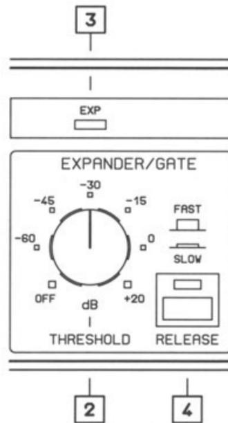
Fig. 12 Control surface of the Expander/Gate section
