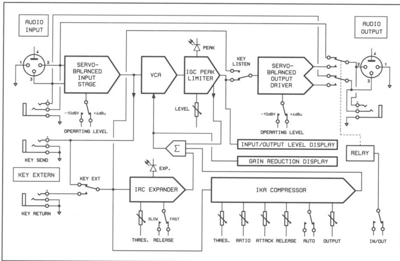
Fig. 3 Block diagram of the Behringer COMPOSER
