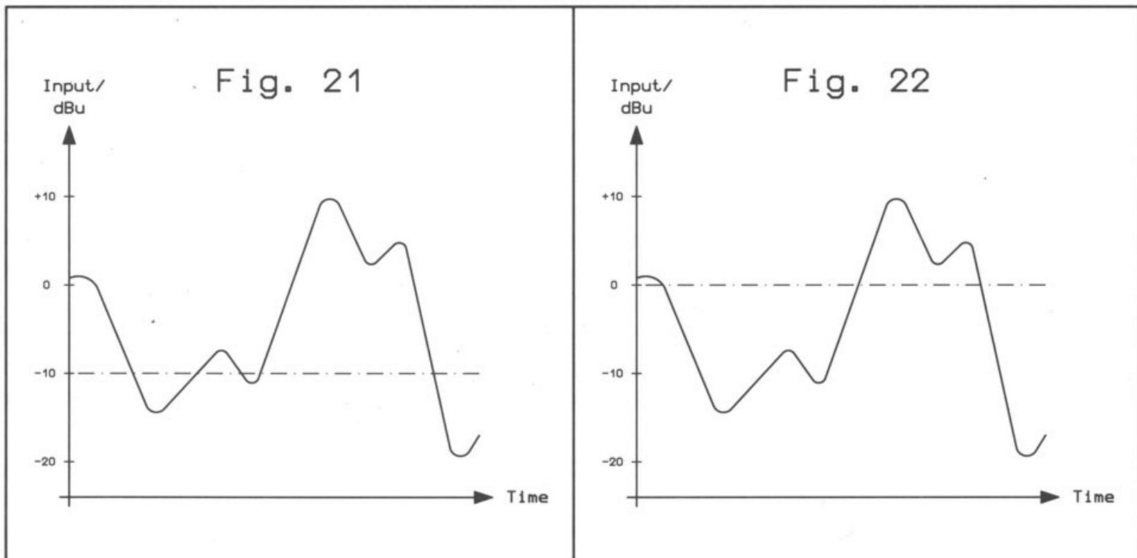
Compressor 1 (fig. 21) and compressor 2 (fig. 22) BEFORE gain control
