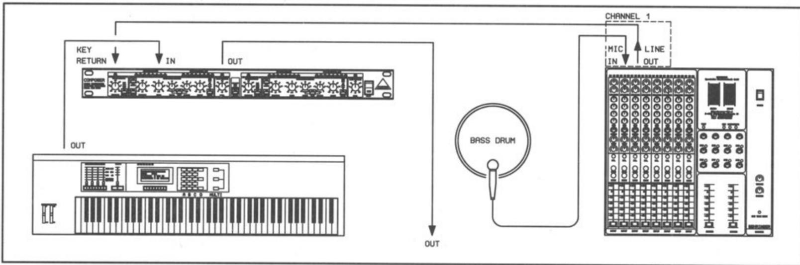
Fig. 38 Triggering a keyboard sound using a bass drum
