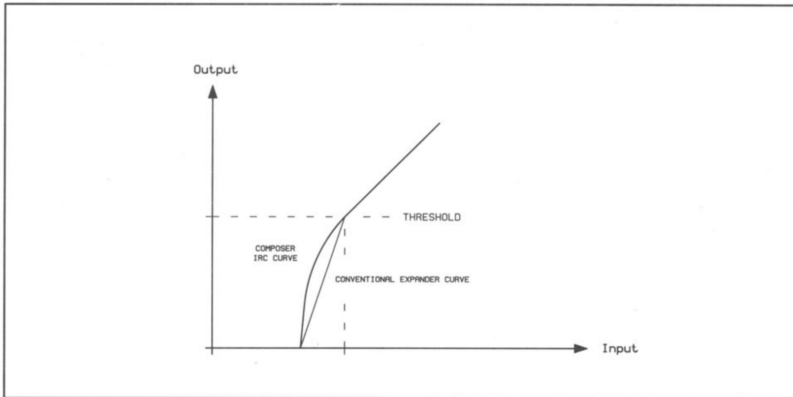
Fig. 17 IRC curve characteristics of the Expander
