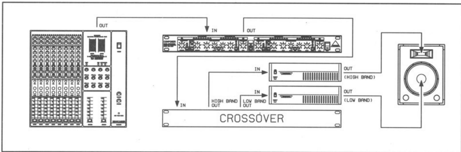
Fig. 31 The Behringer COMPOSER in a two way system
