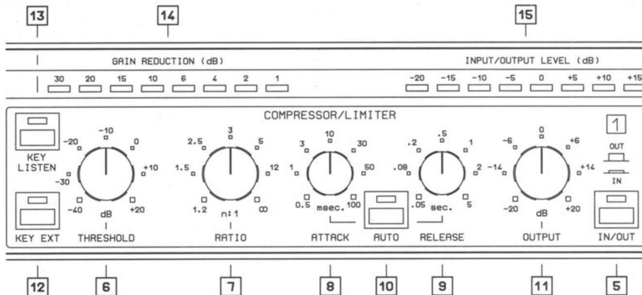
Fig. 13 Control surface of the Compressor section
