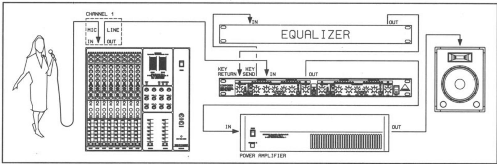
Fig. 35 Reducing feedback in audio systems using the Behringer COMPOSER
