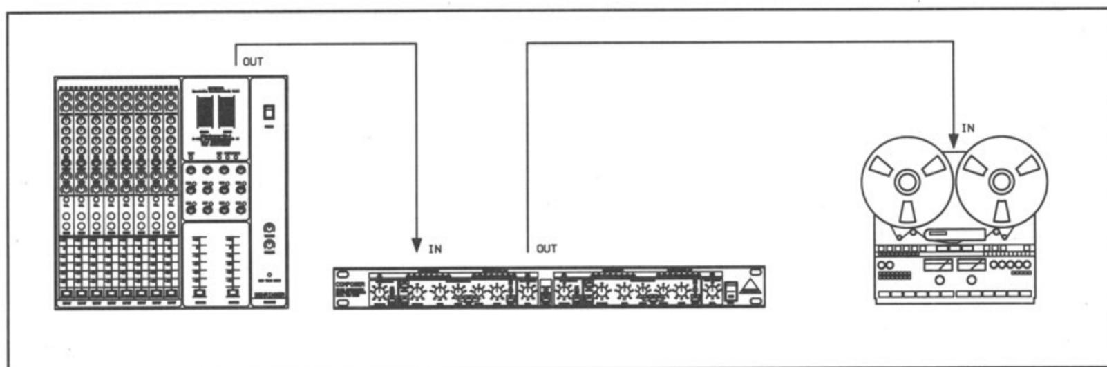
Fig. 33 Using the Behringer COMPOSER to avoid distortion due to tape saturation
