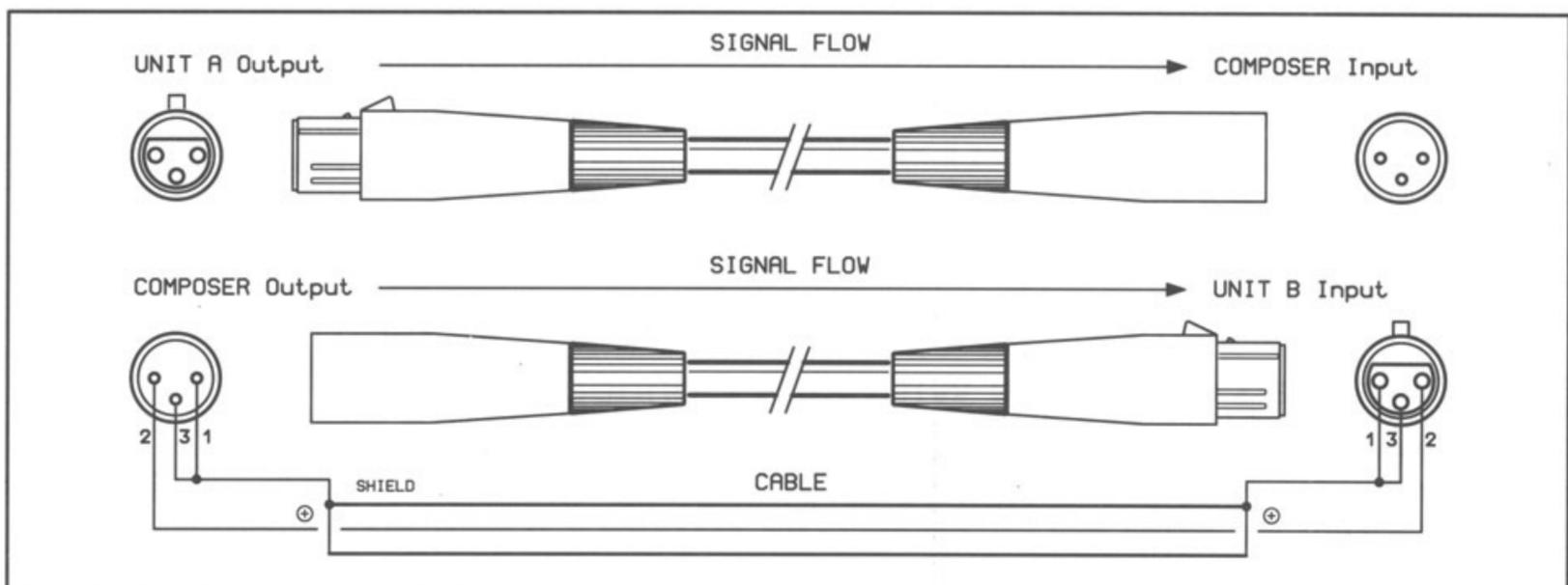
Fig. 7 Unbalanced *input and output wiring* using XLR connectors
