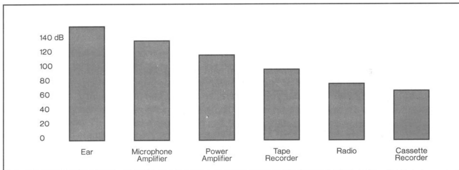
Fig. 1 The dynamic range capabilities of various devices
