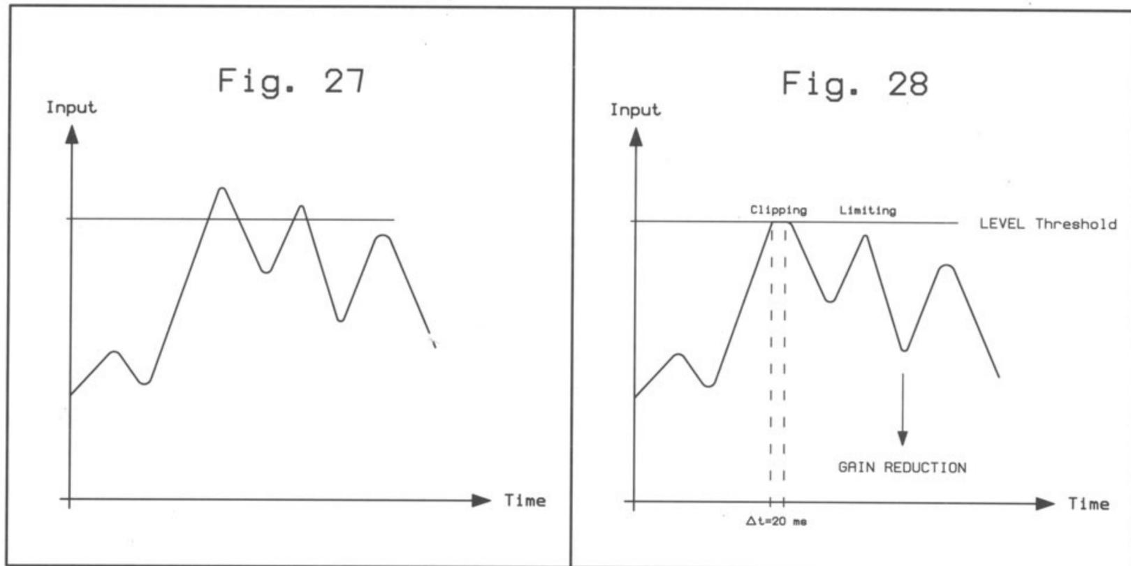
The signal BEFORE gain control (fig. 27) and AFTER IGC peak limiting (fig. 28)
