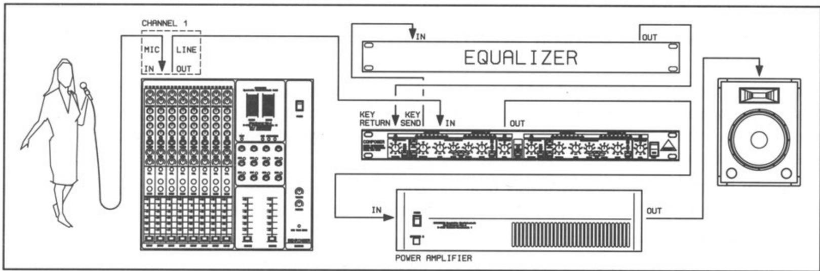
Fig. 34 "De-essing" using the Behringer COMPOSER
