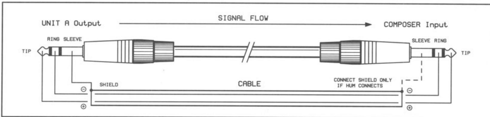
Fig. 8 Balanced COMPOSER *input* wiring with 1/4" jack connections
