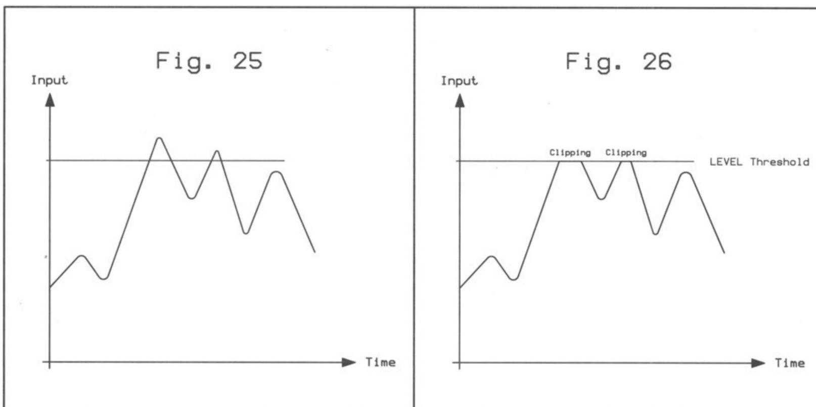
The signal BEFORE gain control (fig. 25) and AFTER clipper processing (fig. 26)
