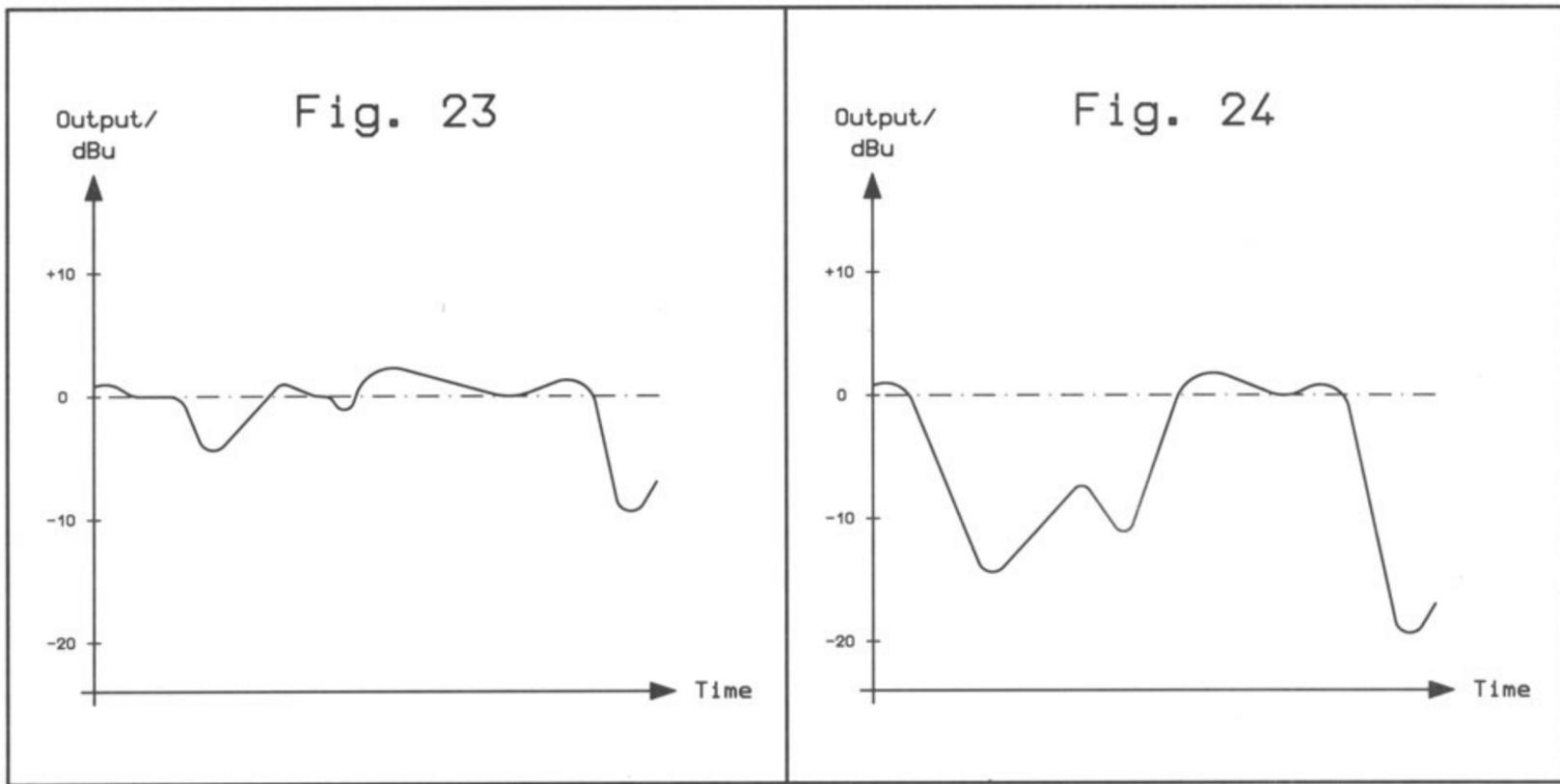
Compressor 1 (fig. 23) and compressor 2 (fig. 24) AFTER gain control
