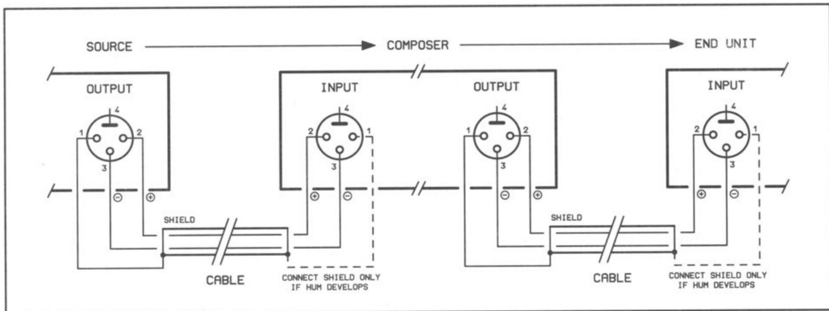
Fig. 4 The correct wiring of the balanced system
