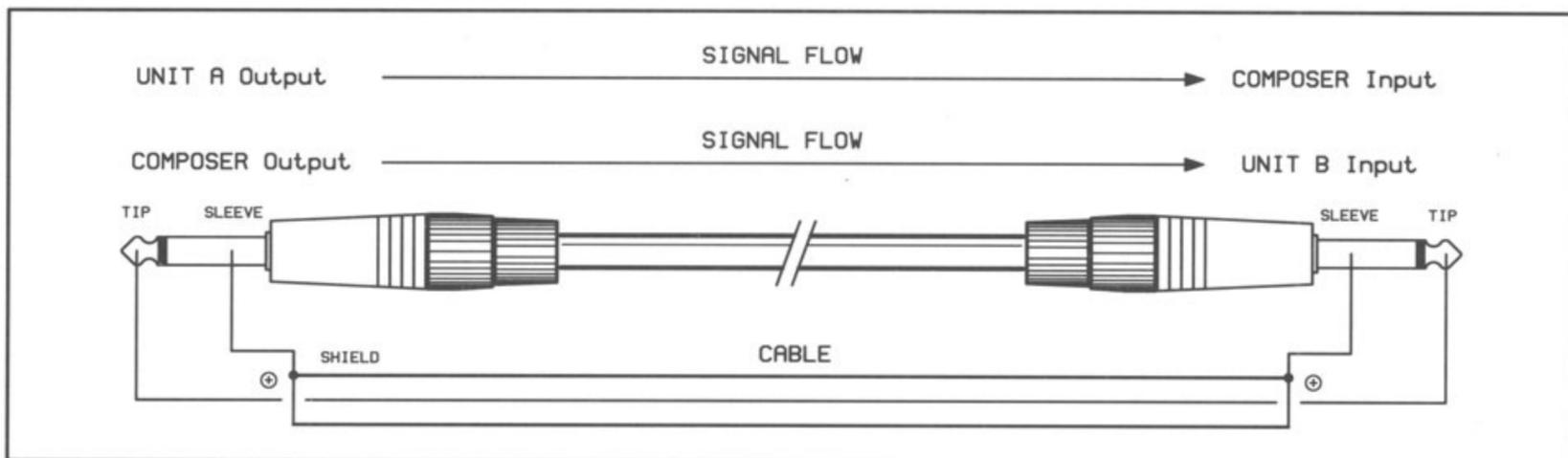
Fig. 10 Unbalanced *input and output* wiring with 1/4" jack connections
