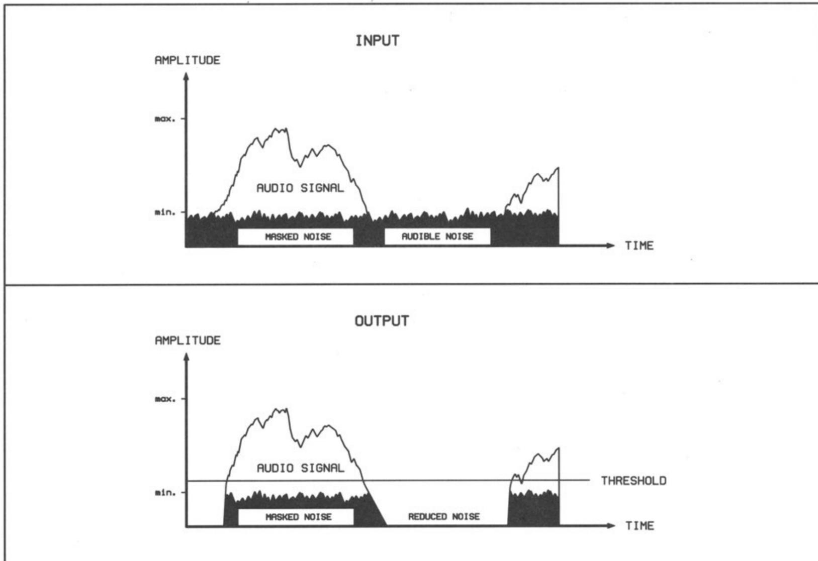
Fig. 16 Function of an expander
