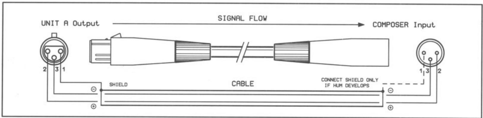
Fig. 5 Balanced COMPOSER *input wiring* using XLR connectors
