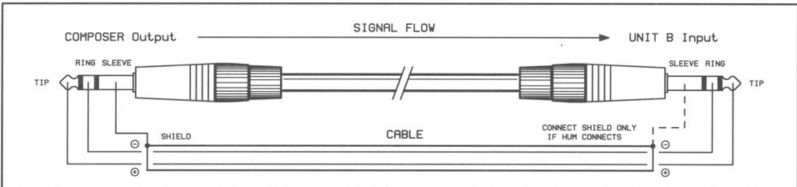
Fig. 9 Balanced COMPOSER *output* wiring with 1/4" jack connections
