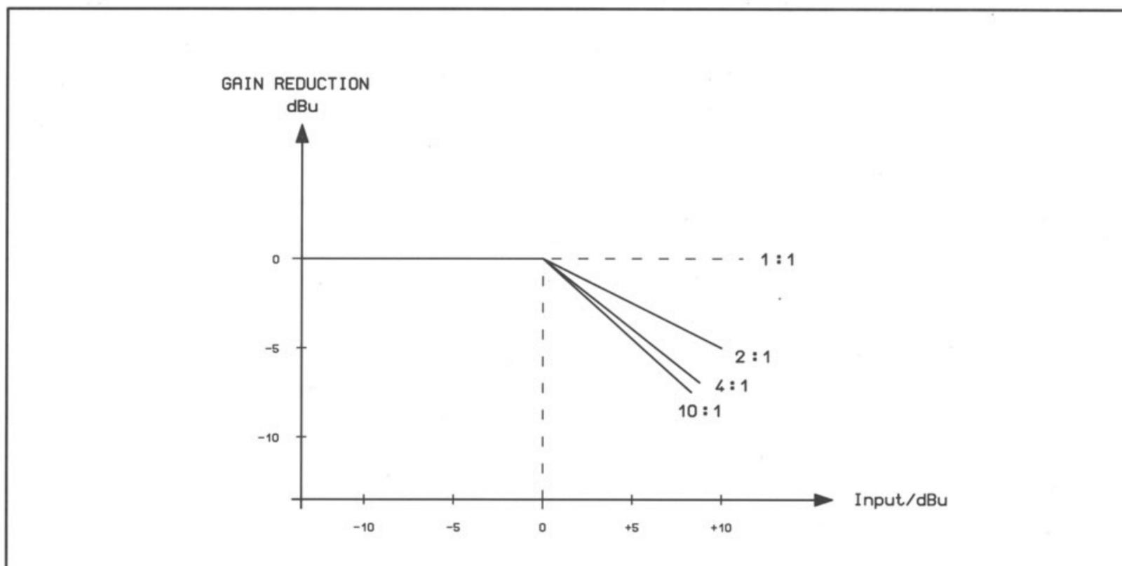
Fig. 20 The effect of a compressor can be expressed as the amount of gain reduction that is taking place for any given input
