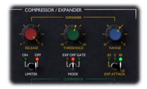
**Release**: Sets how fast the expander drops off when the signal drops below the threshold.
