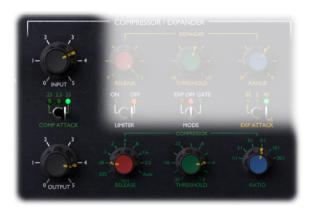
**Input**: This controls the input gain to the compressor circuit. The harder you drive this, the harder the compression will be.
