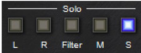
With the **Solo L, R, M and S buttons** you can listen to any element of your stereo mix (stereo signal), mono-ed out (for L, R, M & S), phase-corrected (for “Solo S” only), and on both speakers.
