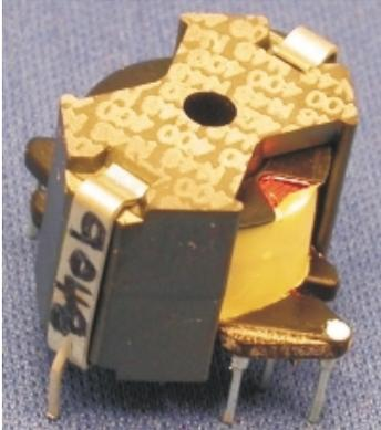
A high performance, professional audio, multi-tapped inductor, intended for line level inductor based equalisation applications.
