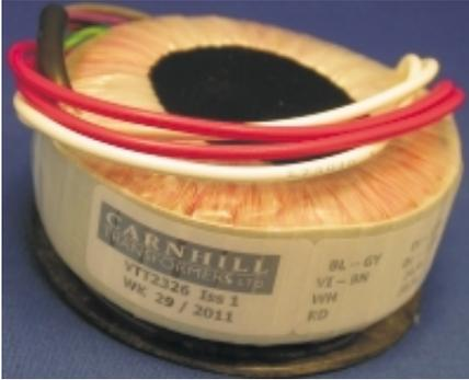
A high performance, no compromise, professional audio power transformer - primarily intended for 24v applications which also require a phantom (+48v) voltage. Fits in a 1U rack enclosure. Dual Primary for 110/120v and 220v/240v usage.
