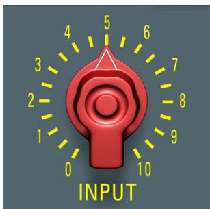
The Input control functions as your input gain/threshold switch which simply drives the Limiter harder as you turn it up. This control emulates the 21-position switch available as a special order option on the Chandler Limited/Abbey Road Special Edition TG1 hardware. Its specially designed taper provides smoother control at lower settings. Crank this up to really hear the unit pump!
