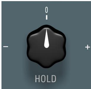
As previously mentioned the Hold control on the 1969 module acts as a back off system to the Limiter side chain. Turning the knob clockwise will give you more gain reduction. You will notice that as the knob is turned to the left the meter rises as the threshold point of the Limiter is reduced. For example if the needle is set at -5 you will have the potential of 8db reduction.
