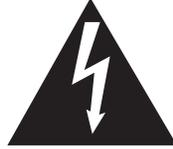
This symbol alerts you to the presence of uninsulated dangerous voltage within the product's enclosure that might be of sufficient magnitude to constitute a risk of electric shock. Do not open the product's case.
