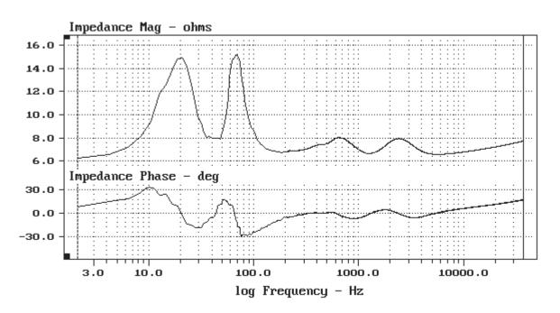
The Sigma 6.2 is a relatively stable load so it is easier for the power amplifier to drive.
