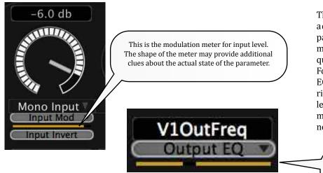
The shape of the meter may provide additional information about the parameter. For example, for a panner the meter is a narrow dot that provides quicker indication of the pan location. For EQ, the meter also reflects the type of EQ—highpass grows downward from the right. Lowpass grows upward from the left. Bandpass has a narrow point marking the passband. Notch has a notch in the solid bar.
