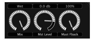
These controls (lower left) allow last-minute adjustment to let a preset fit into your mix. The Mix control should be used when the plugin is inlined. It controls the ratio between wet and dry signal. The Mst Level control overall level, if you need to cut or boost, depending on your material. Mast Fback controls overall feedback of the voices (if feedback levels for any individual values is non-zero).
