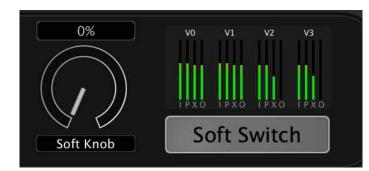
The knob and switch (bottom center of window) are "magic" controls that may be hooked up to control many things in a preset. They're different for every preset, so be sure to try them in every factory preset. They may make small changes or huge changes—and they're automatable. The switch will be highlighted when it's on.
