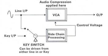
key input. Note that the key input signal is not output from the unit, it is the original input that is compressed, but compression is applied as if the key input signal were being compressed.
