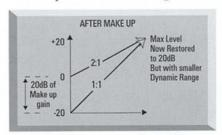
Using the makeup gain restores the volume of the compressed signal.
