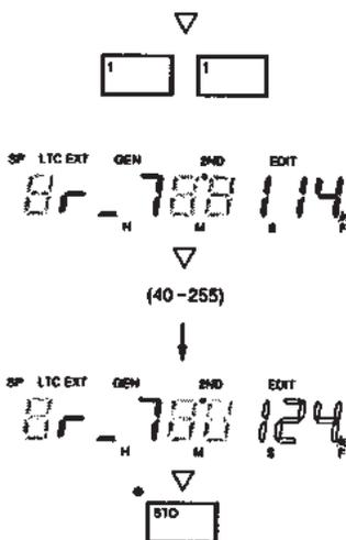
Next, press the [ · ] key. The display will change to "r \_ S 114" (the T will change to S). This indicates that the supply side reel hub inner diameter is registered at 114mm (10 inch reel/default figure). This setup figure can also be changed by the same procedure as that of the takeup reel outlined above. The T (takeup) and S (supply) displays will alternate with each press of the [ · ] key.
