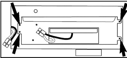
4. Remove the four retaining screws.
