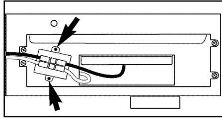
2. Remove the two retaining screws of the cable protection cover then remove the cover.
