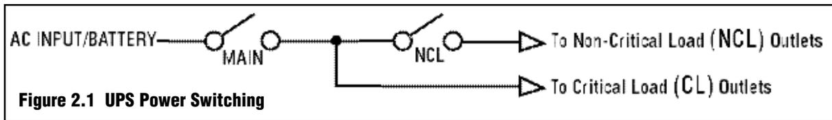
The UPS provides one bank of switched outlets (Outlet Bank 1) that can be controlled independently. These are referred to as Non-Critical Load (NCL) Outlets.
