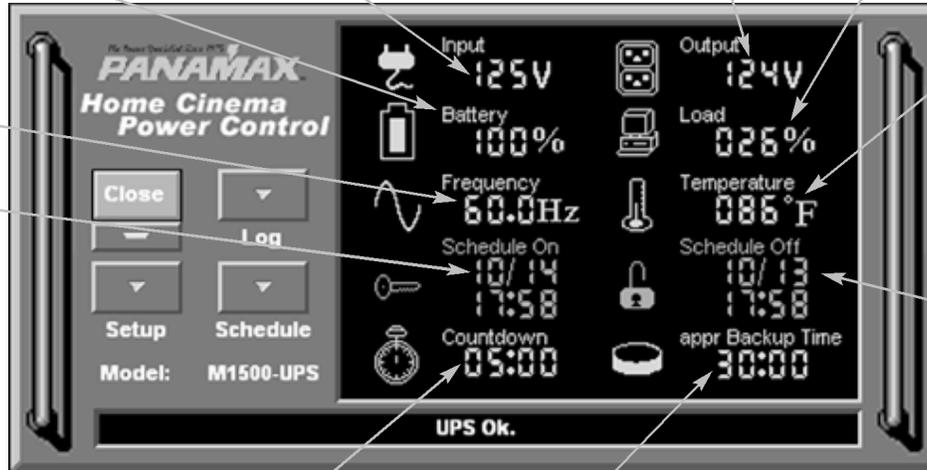
**5. Temperature:** Displays the internal operating temperature of the unit. If the temperature exceeds 158°F (70°C), the indicator will change from green to red.
