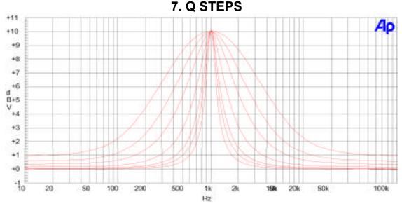
A range of Q values and its graphical representation are illustrated in this plot. The actual Q characteristic supported by the Model 8200 is continuously variable, though this plot merely represents a few stepped increments. Q values are variable from 0.4 (broad Q) to 4.0 (sharp Q) on each band, with the addition of counter-clockwise detents for shelving characteristics on both the Low and High bands of each channel.
