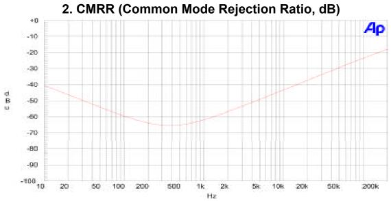
This plot depicts the relationship between CMRR level (dB, along the left axis) and frequency (Hz, along the bottom axis). In this test, a +20 dBu sine signal was swept from 200 kHz to 10 Hz in 500 steps.
