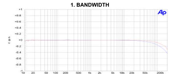
As can be seen in this plot, the bandwidth of the Model 8200 is quite extended and extremely flat. Notice that the limits of the plot along the left axis are +/- 1.0 dBu. The blue line represents the 'EQ Out' state, while the red line graphs the 'EQ In' state. Refer to the Specifications page of the Model 8200 User's Manual for more detailed bandwidth measurements.
