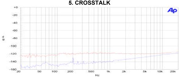
This plot illustrates the inter-channel crosstalk specification of the Model 8200. The blue line represents the 'EQ Out' state, while the red line represents the 'EQ In' state. A +20 dBu swept sine test signal was used to generate these results. Measurement was taken from the output of the right channel, with the left channel receiving the signal and the right input grounded.
