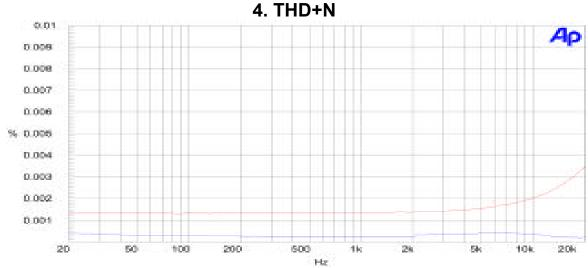
Total Harmonic Distortion (plus noise) is examined in this plot, in both the 'EQ Out' (blue) and 'EQ In' (red) states of operation. This test was conducted with a +20 dBu swept sine waveform from 20 kHz to 20 Hz. It can clearly be seen that the distortion content is very low in both states--this quantitative analysis is indicative of the widely touted qualitative conclusion regarding the transparency of the Model 8200.
