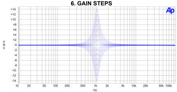
This plot elucidates the range of gain and attenuation available on each band of the Model 8200. Although the graphic depicts gain steps, the actual gain characteristic offered by the Model 8200 is continuously variable from -15 dB to +15 dB, with a highly accurate 0 dB position (no detent).
