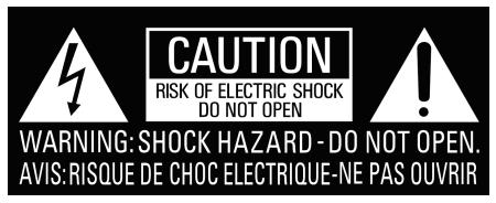
The lightning bolt with arrowhead symbol within an equilateral triangle is intended to alert the user to the presence of uninsulated "dangerous voltage" within the product's enclosure that may be of sufficient magnitude to constitute a risk of electric shock to persons.
