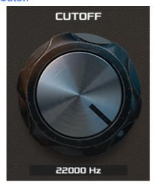
Every DJ's favorite knob - use this to adjust the specific frequency at which the filter is centered. We made this one bigger so you don't grab the wrong one by accident.;)
