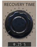
Adjusts the Recovery Time (also known as release in many other compressors) in seconds.
