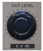
Adjusts the final output gain level of the compressor (also known as makeup gain.)
