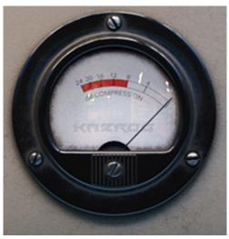
A vintage-style meter showing the current amount of compression. Accurate within +/- 3 dB, this meter is not intended for modern loudness calibration, really just here to give visual feedback (and look cool.)
