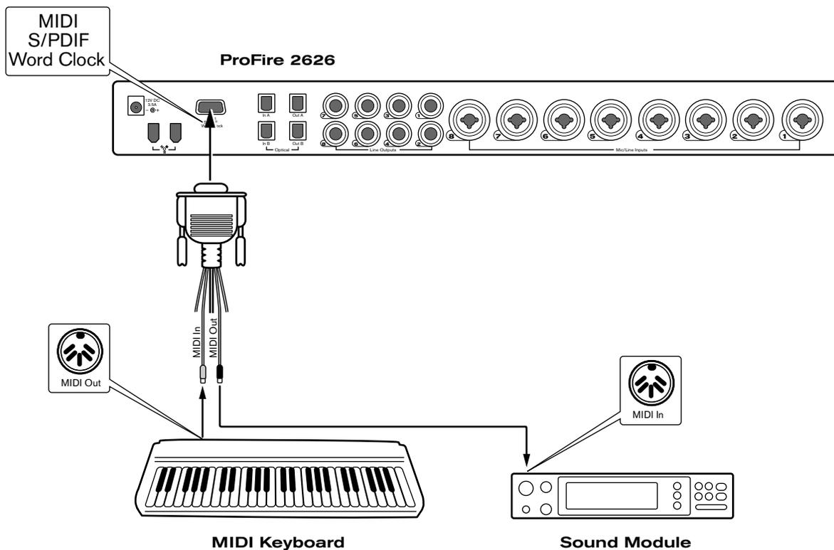
1. Make sure the breakout cable is connected to the back of ProFire 2626.
