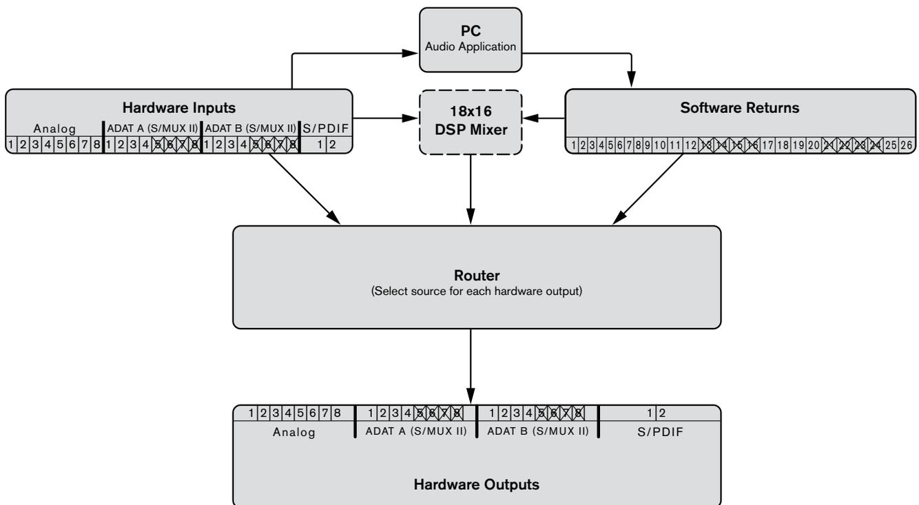
At sample rates of 88.2 or 96 kHz, the ADAT ports operate in S/MUX II mode. As a result, the number of available ADAT channels is reduced to four channels per port (i.e., channels 5-8 are disabled on all ADAT I/O ports) and software return channels 13-16 and 21-24 are disabled.
