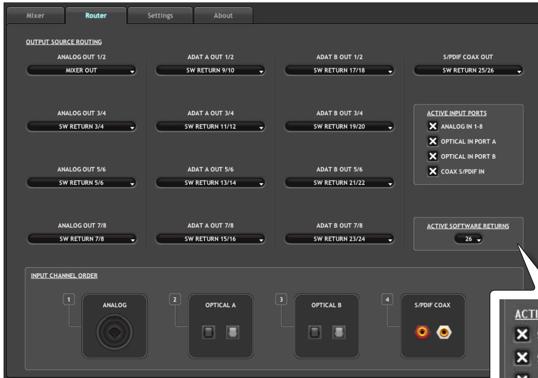
The ProFire 2626 Router tab contains a variety of parameters affecting how audio is routed through the interface. These parameters are grouped into categories as explained on the following pages.
