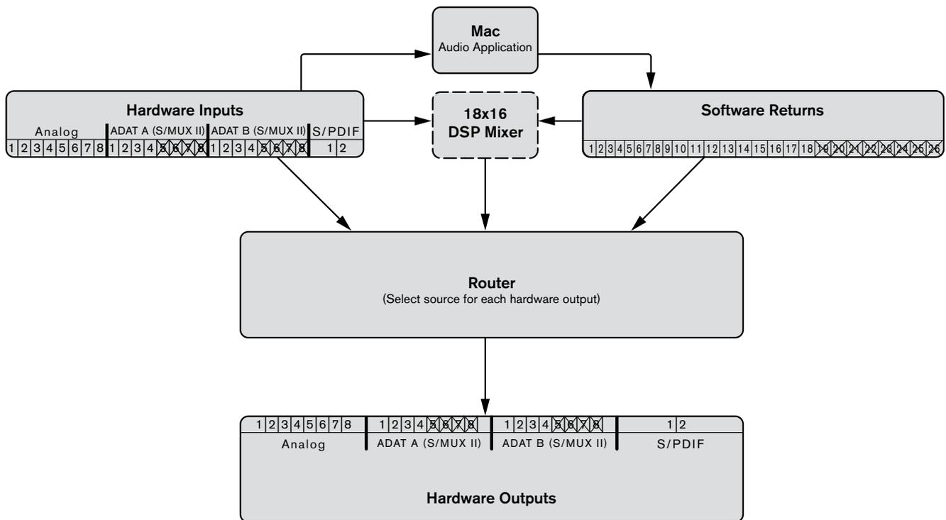
At sample rates of 88.2 or 96 kHz, the ADAT ports operate in S/MUX II mode. As a result, the number of available ADAT channels is reduced to four channels per port (i.e., channels 5-8 are disabled on all ADAT I/O ports) and software return channels 19-26 are disabled.
