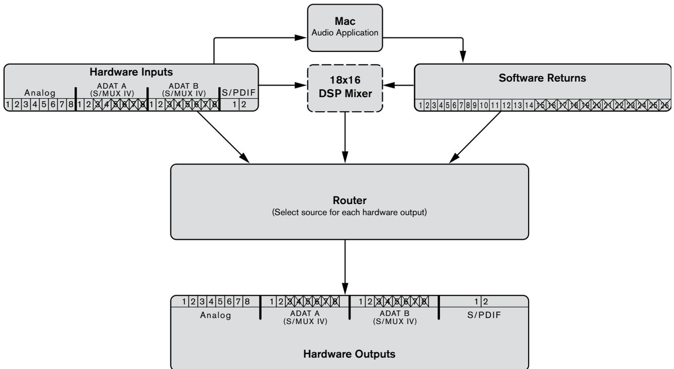
At sample rates of 176.4 or 192 kHz, the ADAT ports operate in S/MUX IV mode. As a result, the number of available ADAT channels is reduced to two channels per port (i.e., channels 3-8 are disabled on all ADAT I/O ports), and software return channels 15-26 are disabled.
