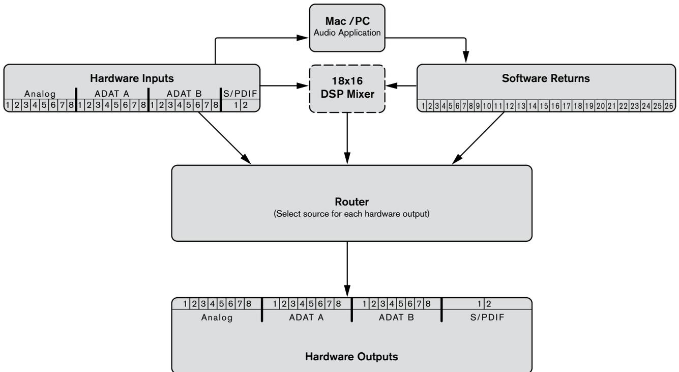
**Hardware Inputs** – These are the physical audio inputs on ProFire 2626 including the eight analog combo jacks, two instrument inputs, two ADAT ports, and the S/PDIF connector. All signals that enter the interface through the hardware inputs can be sent to the Mac/PC, DSP Mixer, and Router (all described below).
