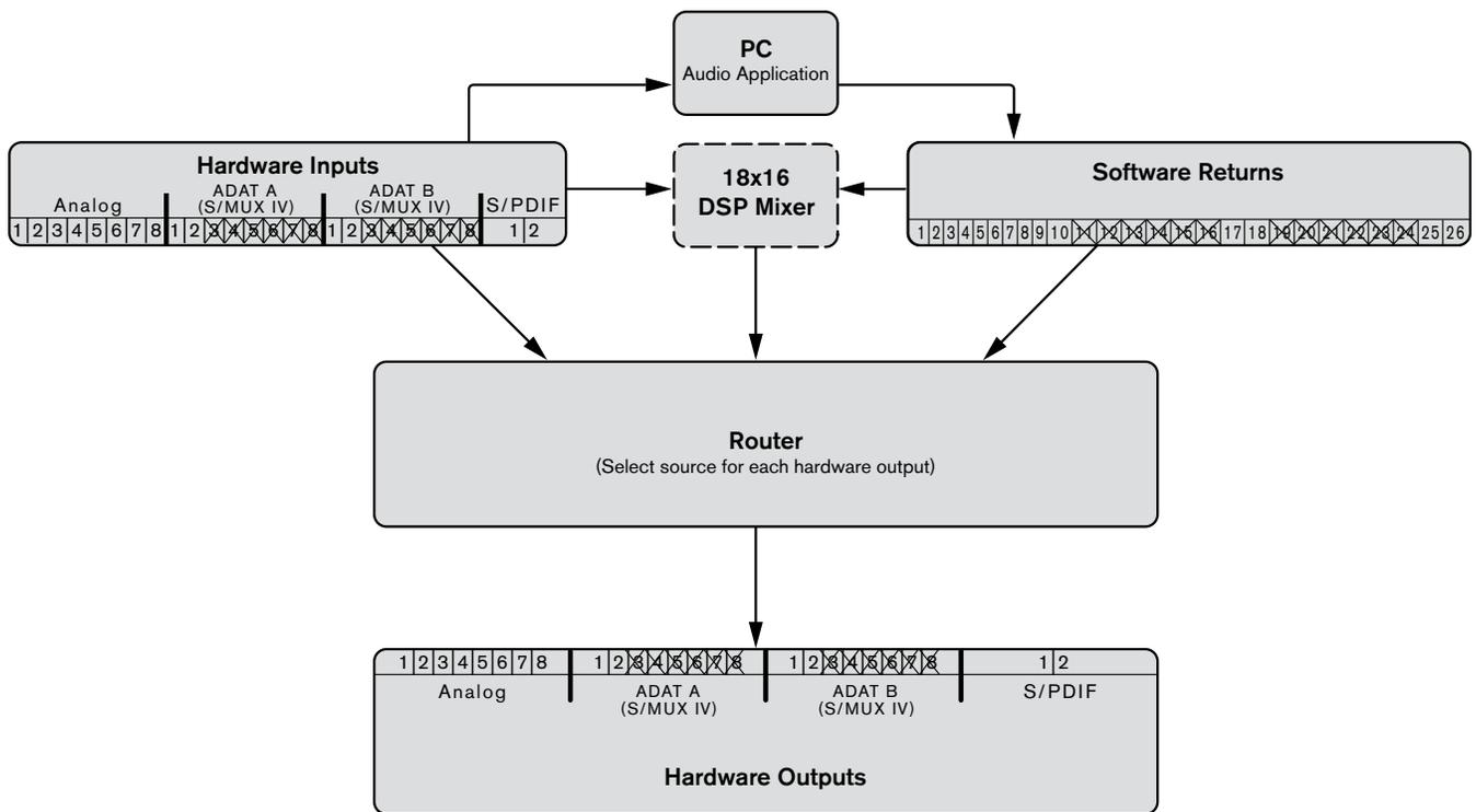
At sample rates of 176.4 or 192 kHz, the ADAT ports operate in S/MUX IV mode. As a result, the number of available ADAT channels is reduced to two channels per port (i.e., channels 3-8 are disabled on all ADAT I/O ports), and software return channels 11-16 and 19-24 are disabled.
