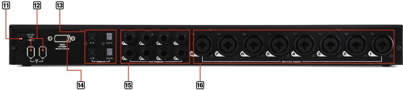
11. **Power Supply Connector:** Connect the included power supply here. Use only the power supply provided with the interface or an equivalent power supply with the same rating and polarity.
