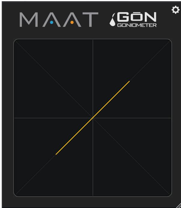
*Figure 2 - A hard-panned mono input produces a variable length line at  $45^\circ$*
